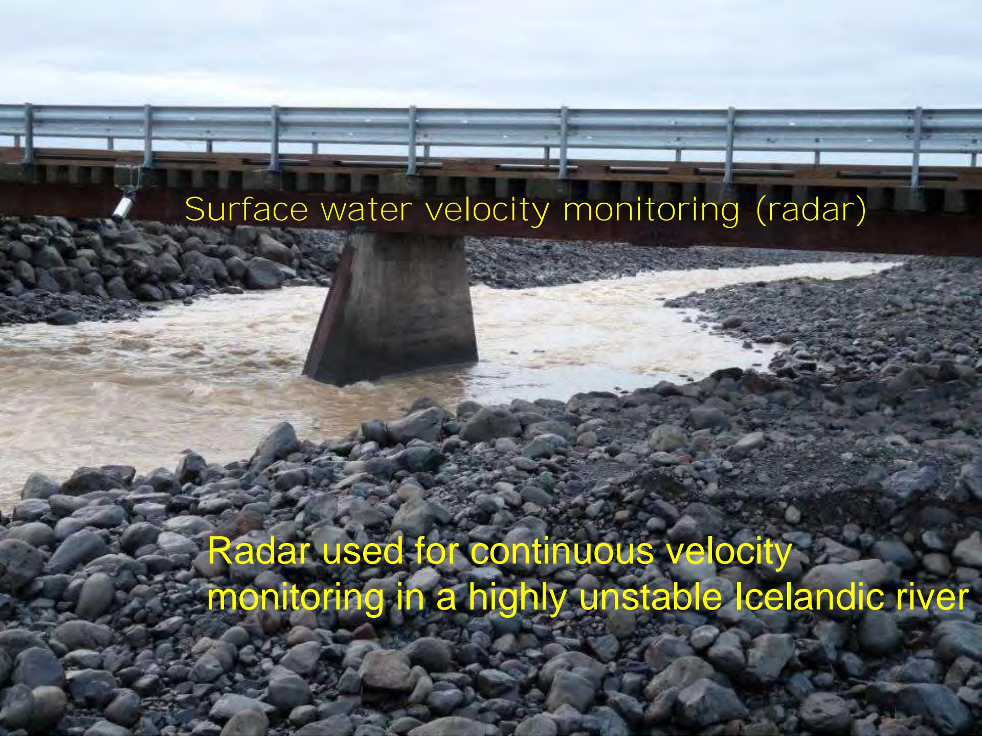
Surface water velocity monitoring (radar)
